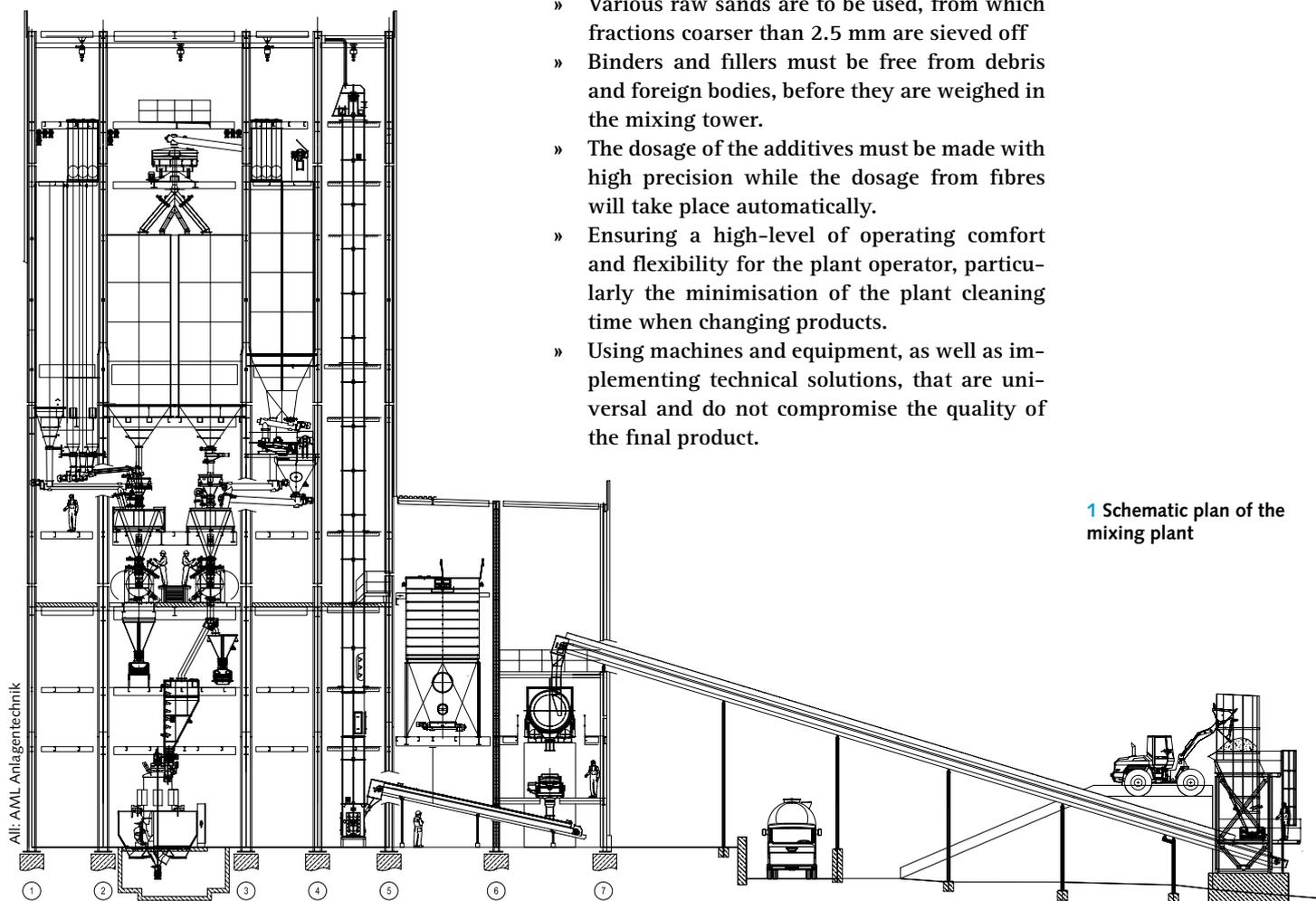
1 Schematic plan of the mixing plant
