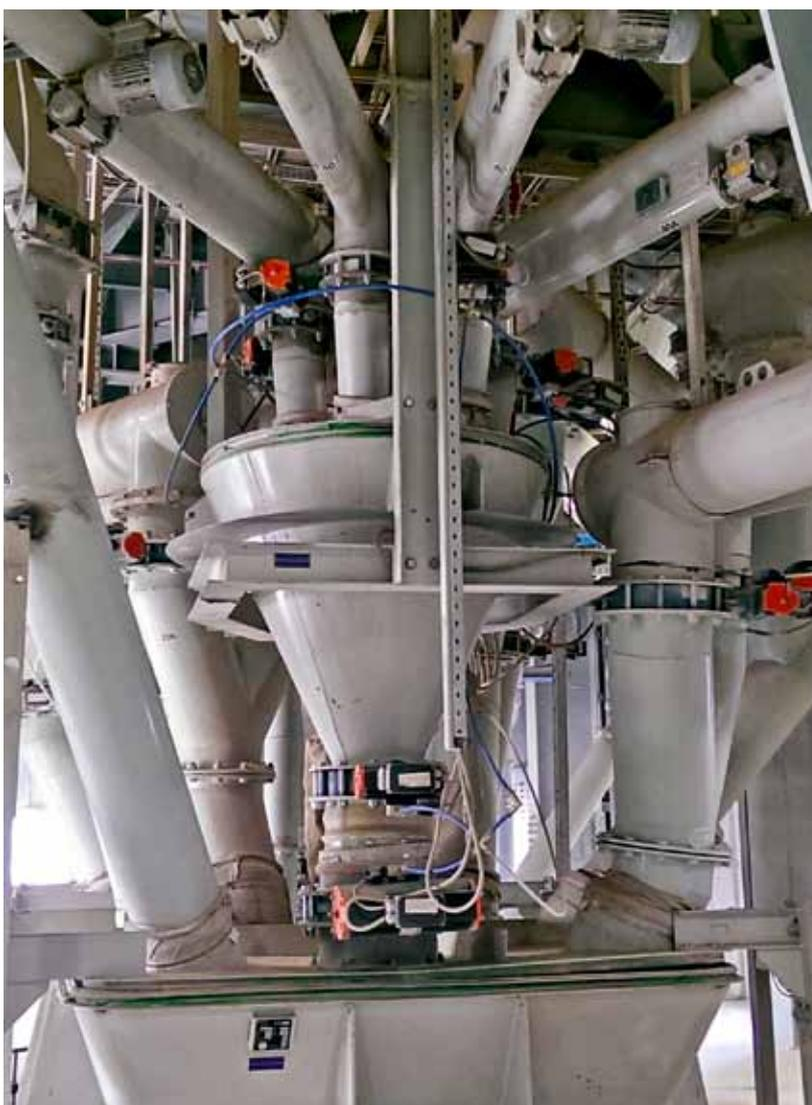
the raw material. Freed from any foreign bodies and unwanted oversized grains, the raw materials are stored in technological hoppers and afterwards dosed into the main weighing hopper via screw conveyors. The use of this method is indispensable for the production of finer products like fillers, grout and adhesives.
